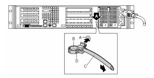
Figure 15: Installing the Power Cord
